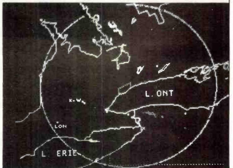
Below: The same image with clutter elimination circuit operating.
